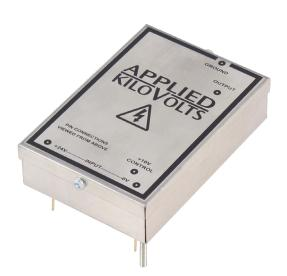
This range of power supplies are miniature versions of the HP family giving up to 1kV, 2.5kV, or 3kV, at 2W. The units, which are programmable by a 0 to +10 volt signal, are intended to be mounted on a printed circuit board and offer high stability together with low drift. They use high frequency pulse width modulated switching techniques in conjunction with a ferrite step-up transformer to control the output voltage.
