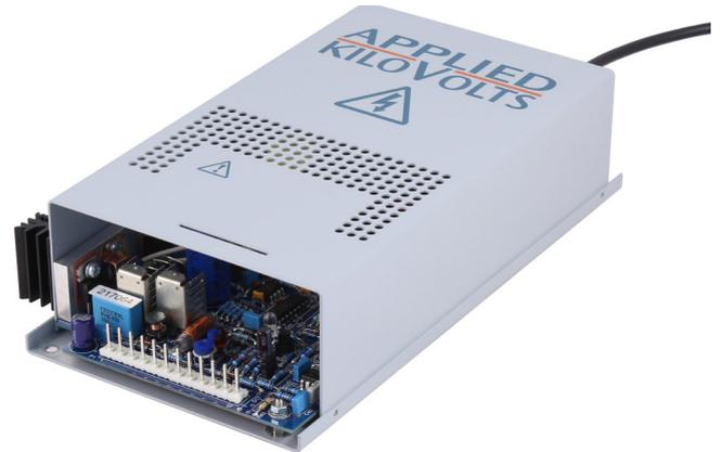
The HW series of high voltage modules covers the range from 1kV to 50kV giving 100 watts of output power. Control of the output voltage is by internal potentiometer or by external potentiometer or by an external 10 volt analogue control voltage. Pins 1 to 10 of the 12 pin Molex input connector are pin compatible with both the high precision HP series and the general purpose KS series (please see separate data sheets).
