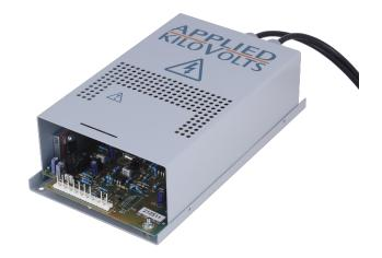
These power supplies are intended to power microchannel plate and imaging detectors, that are isolated by many kV from ground. They give 0 to +3.5 kV and can be floated on voltages up to ±2.5 kV (HFxx2.5), ±10 kV (HFxx010), ±20 kV (HFxx020) & ±30 kV (HFxx030).
