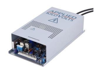
These power supplies use the proven power oscillator from the standard 100 watt HW series and are intended to power ion gun, electron gun & X-ray filaments of up to 1.5 ohm (including cable resistance). The filaments can be isolated from ground by up to 30 kV, while power input & all controls remain at ground potential. O/P current from 0.8A to 5A is current controlled. Higher isolation voltages are also possible. Please consult the factory for more details.
